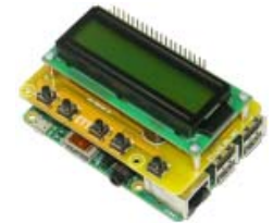
Figure illustrates the connection between Board ET-LCD SW HAT and Board RASPBERRY PI.
